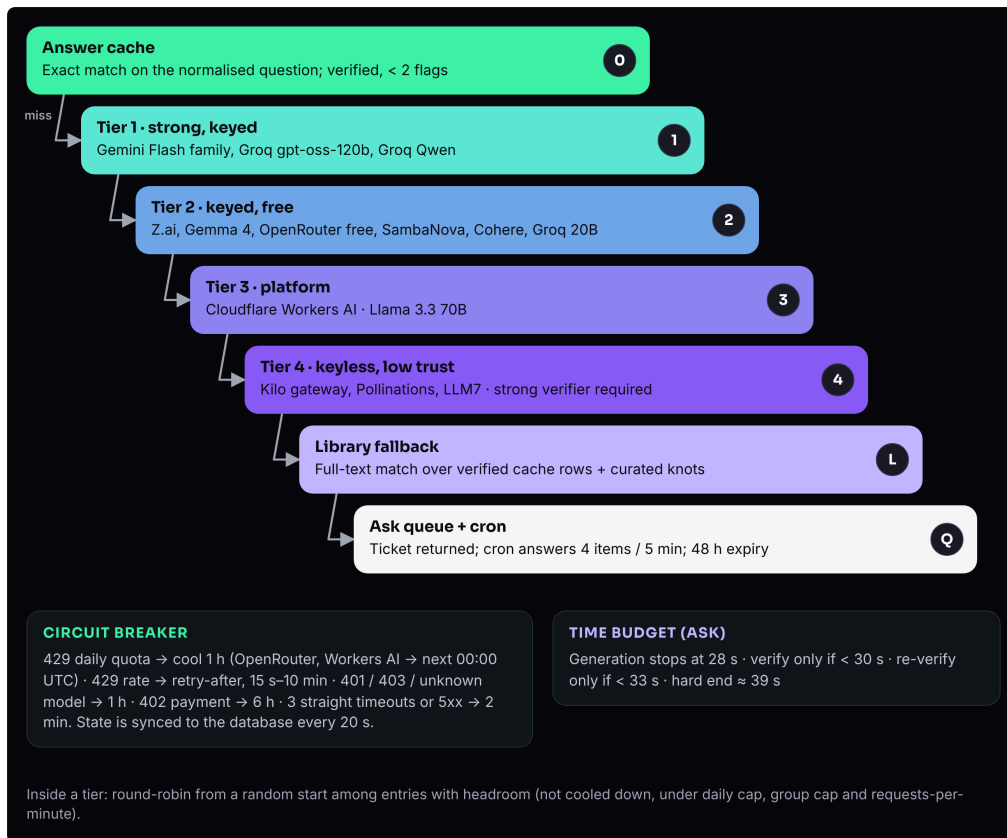
Figure 5.6. Request failover cascade from cache to provider tiers, library and queue, with circuit-breaker rules and the time budget.
